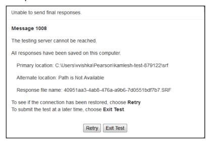
This message appears if the connection with the testing server and TestNav was unable to upload responses to the testing server. As the message indicates, the student responses have been saved locally (e.g., to a local drive or network drive) so that they can be uploaded to the Pearson server when connectivity has been restored.
