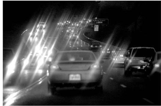
the BGE method described on page 7. Dirt on the windshield also causes glare, as dirt on glass reflects rays of light, either from the sun or headlights.
